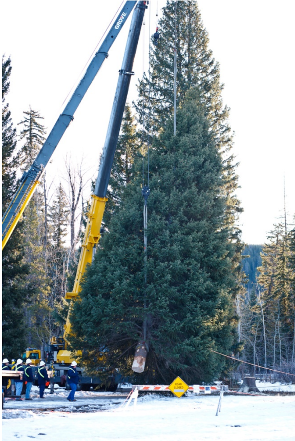
CAPTION: Before the Tree was cut, it was suspended by a crane so that it could be lowered safely onto the truck.
